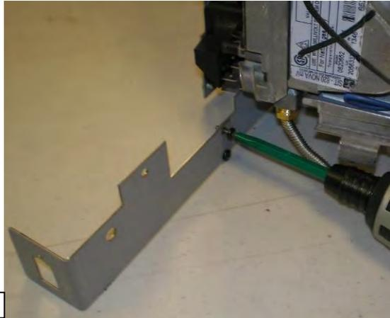
**2** Attach On/ Off Switch Extension Bracket using [2] #6 Combo Screws as shown.
