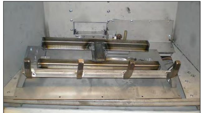
**Step 2:** Locate and remove the twelve [12] screws around the outside of the burner pan. This will remove the entire burner assembly.
