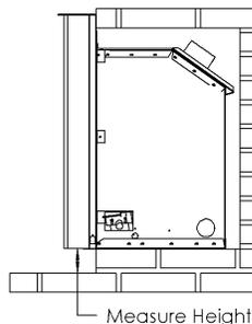
Fig. 2 - Front view with Riser Kit.
