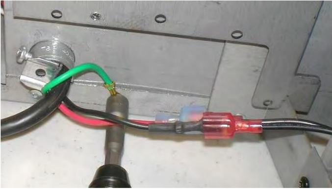
**NOTE:** If Ground is attached to Side Component Plate, remove and fasten to side of appliance with a DT Screw.
